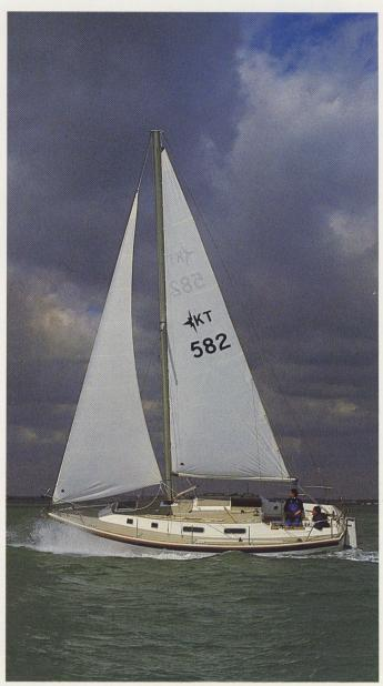
**The Rig** A single spreader masthead rig with a deck stepped mast. All standing rigging is stainless steel with prestretched Terylene running rigging.
