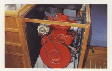
**Engine** Konsort is powered by a well known 18hp twin cylinder diesel engine, which drives the boat quietly and economically at over six knots through a conventionally driven two-bladed propeller. The engine is fitted with decompressors and provision for hand-starting. The sounddeadened engine compartment is designed to give maximum access for routine maintenance.
