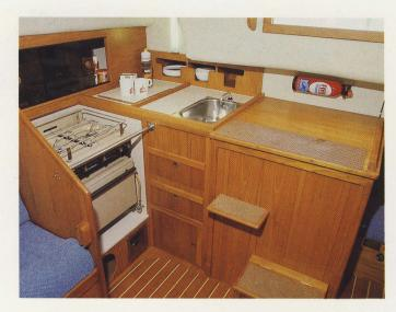
There is a large stainless steel sink supplied from a 30 gallon stainless steel fresh water tank.
