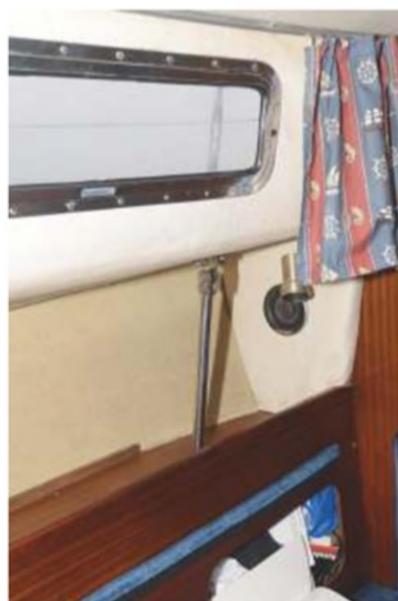
The interior fit-out allows easy access to the shroud chainplates
