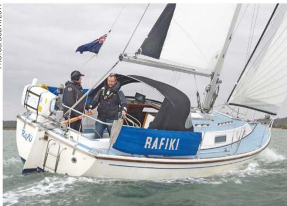
ABOVE: A transom-hung rudder is simple, robust and easier to fix than a through-hull rudder stock if it breaks
