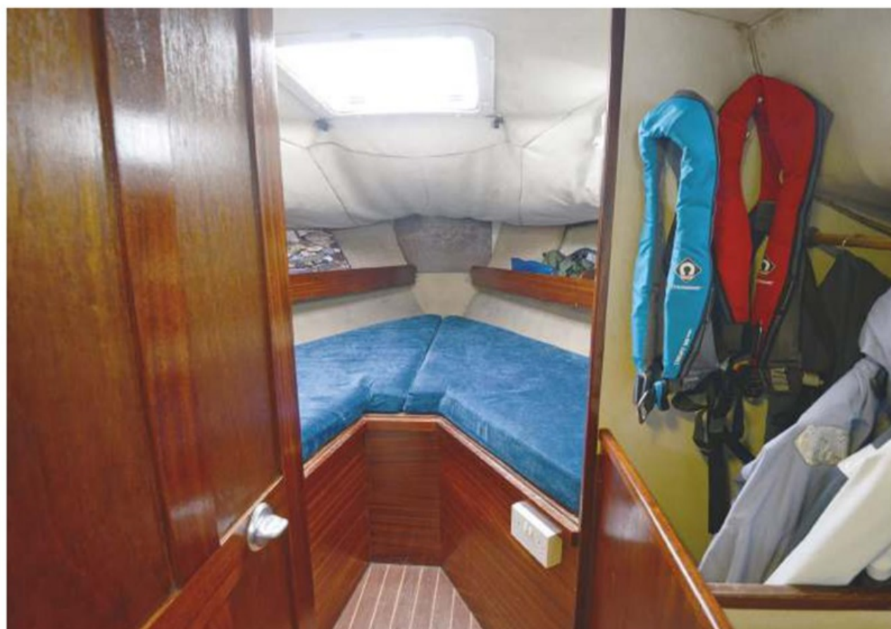
There's a wet locker opposite the heads. Note the sagging headliner in the forecabin
