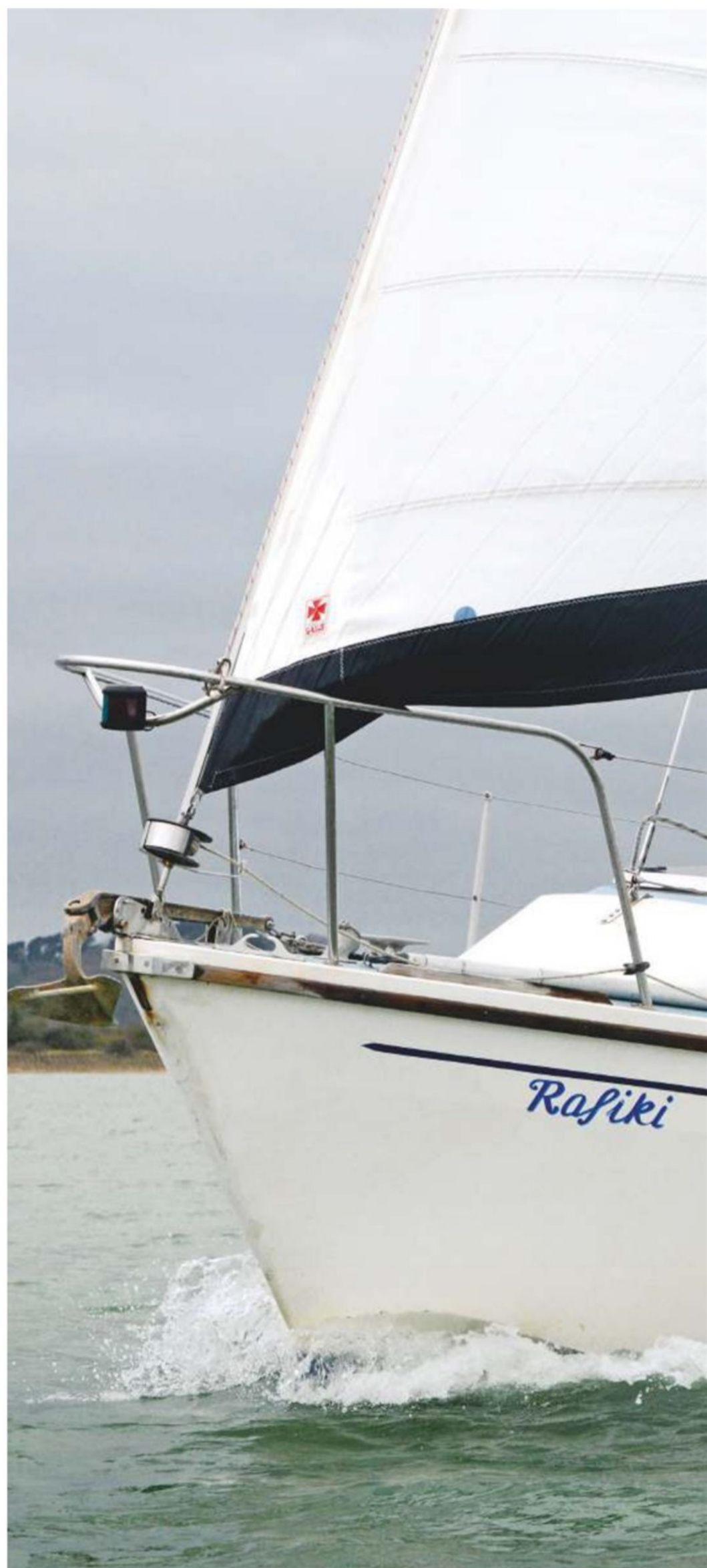
ABOVE: A transom-hung rudder is simple, robust and easier to fix than a through-hull rudder stock if it breaks
