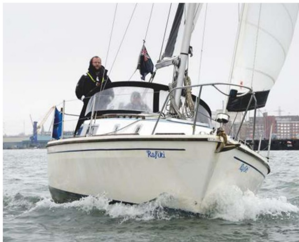
A fine bow chine high in the topsides is designed to deflect waves
